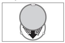
The roasting filter must be fitted in front of the fan when cooking anything fatty, or where food is likely to splatter, e.g. when open roasting or grilling meat.
